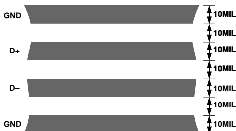
Figure 18. Arrangement of Signal Tracks
