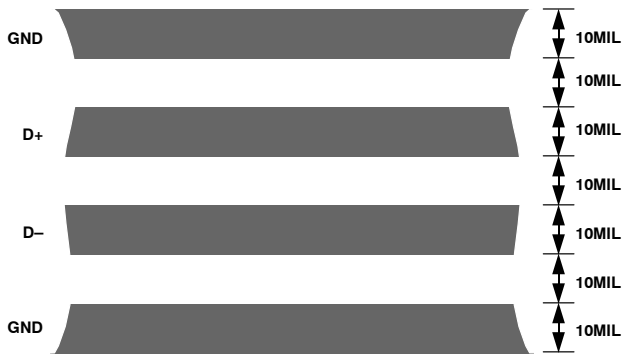
Figure 18. Typical Arrangement of Signal Tracks
