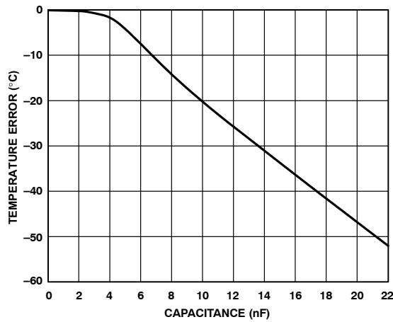
Figure 3. Temperature Error vs. Capacitance Between D+ and D-
