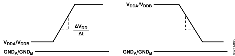
Figure 13. Transient Immunity Waveforms—Output Supplies
