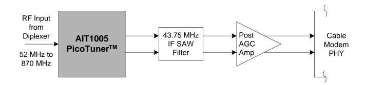
Figure 1: Tuner Downstream Path
