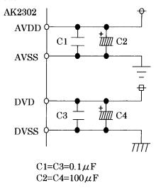
To use the same supply for both digital and analog power supply (DVDD and AVDD), insert  $10\Omega$  resistor between AVDD and DVDD. AVSS and DVSS must be separated on the board, and connected them at power supply unit.
