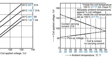
Pick-up and drop-out voltage, V
