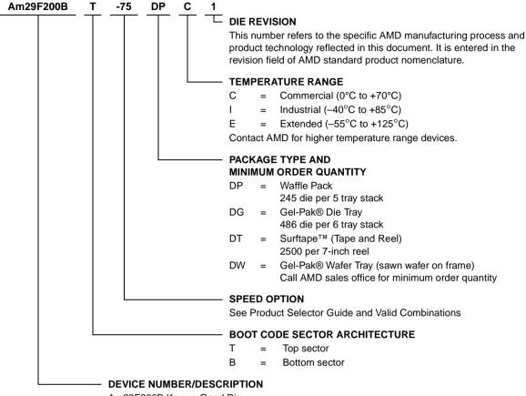
Am29F200B Known Good Die 2 Megabit (256 K x 8-Bit/128 K x 16-Bit) CMOS Flash Memory—Die Revision 1 5.0 Volt-only Program and Erase
