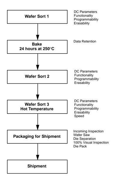
Figure 1. AMD KGD Product Test Flow
