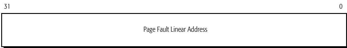
Figure 23. Control Register 2 (CR2)
