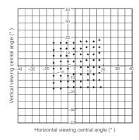
(2) Each pixel's viewing angle (half angle) Central 4 pixels (Pixel No. 28, 29, 36, 37) viewing angle (half angle): horizontal direction Typ. 5.0 ° vertical direction Typ. 4.7 °
