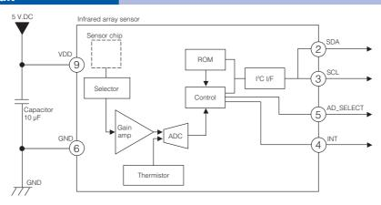
\* INT terminal 4 normally has same voltage as VDD. When interrupting, same as GND (0V)
