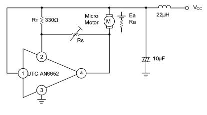
$\begin{cases} \text{Ka:Generation constant=2.4mV/rpm} \\ \text{Ra:Internal resistor = } 18\Omega \\ \text{KT:Torque constant=200g} \cdot \text{cm/A} \end{cases}$
