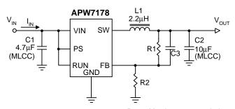
$R1 \le 1M\Omega$  is recommended  $R2 \le 200 K\Omega$  is recommended
