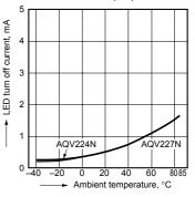
9. Off state leakage current Sample: AQV227N, AQV224N; Measured portion: between terminals 4 and 6; Ambient temperature: 25°C 77°F
