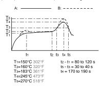
Temperature rise of relay itself may vary according to the mounting level or the heating method of reflow equipment. Therefore, please set the temperature of soldering portion of relay terminal and the top surface of the relay case not to exceed the above mentioned soldering condition. It is recommended to check the temperature rise of each portion under actual mounting condition before use.
