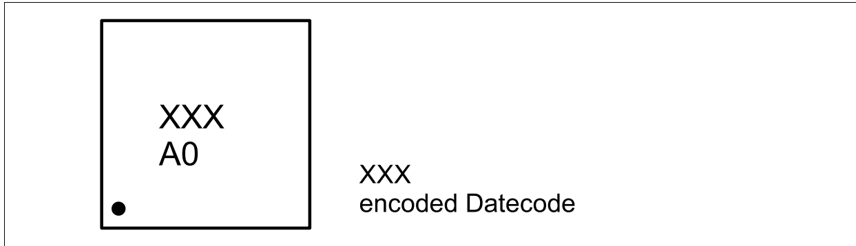
Figure 12. 8-pin MLPD (2x2mm) Marking
