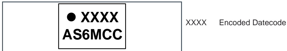
Figure 37: WLCSP Package Marking/Code
