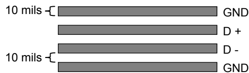
Figure 11. Recommended Remote Diode Circuit Board Interconnect
