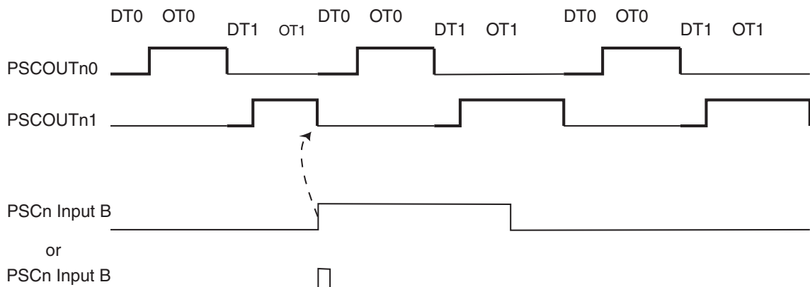
Figure 12-34. PSC behavior versus PSCn Input B in Mode 8
