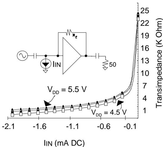
Figure 8: Transimpedance vs. I<sub>IN</sub>
