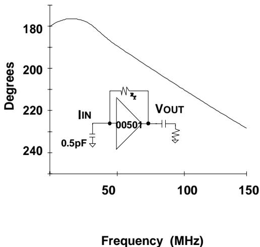
Figure 14: Phase ( $I_{IN}$  to  $V_{OUT}$ )
