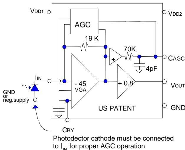
**Figure 1: Equivalent Circuit**
