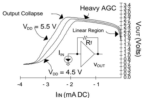
Figure 10: V<sub>OUT</sub> vs. I<sub>IN</sub>
