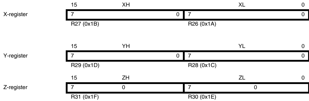
Figure 7-3. The X-, Y-, and Z-registers
