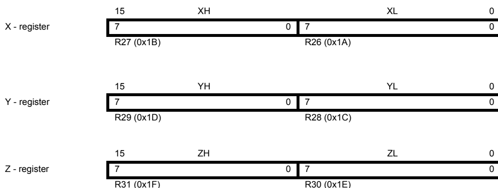
Figure 6-3. The X-, Y-, and Z-Registers
