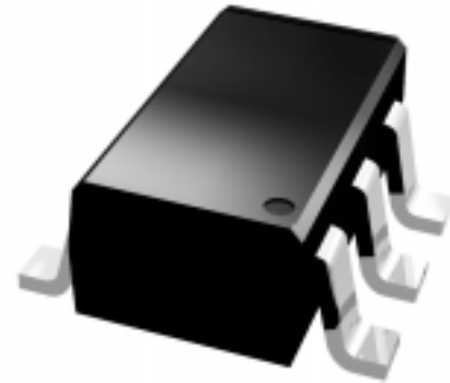
S14 SOT-6 6 Pin Plastic Package
