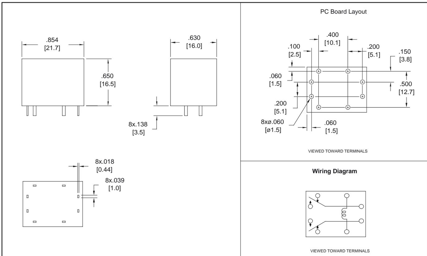
Dimensions in inches with metric equivalents in parentheses. Tolerance:  $\pm .010$ "
