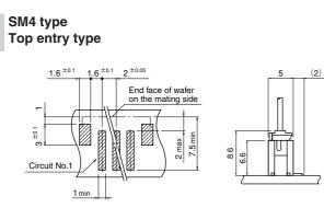
Note: 1. Tolerances are non-cumulative: ±0.05mm for all centers. 2. The dimensions above should serve as a guideline. Contact JST for details.
