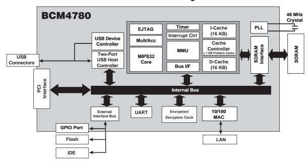
The Broadcom NASoC **BCM4780P** processor is a high-performance, low-power chip designed for low and medium NAS products.
