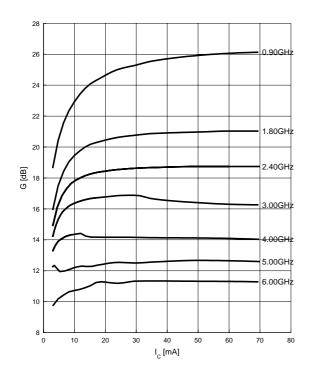
Power gain  $G_{ma}$ ,  $G_{ms} = f(f)$  $V_{CE} = 3 \text{ V}$ ,  $I_{C} = 60 \text{ mA}$
