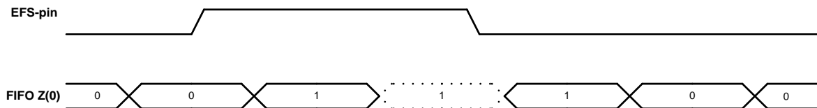
Timing diagram for external FIFO synchronization. EFS-pin is the Interrupt pin configured as EFS-Mode. FIFO z(0) is the least significant bit of the z-axis gyro data stored in the FIFO.
