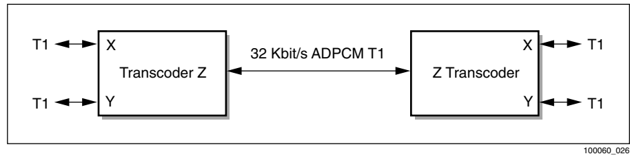
Figure D-2. Single-Board Transcoder Application
