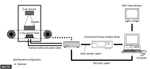
• The C7390 X-ray line sensor camera consists of a sensor head, sensor control unit and cables. Image display equipment should be ordered separately.
