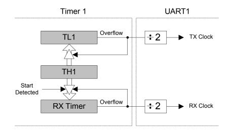
Figure 23.2. UART1 Baud Rate Logic
