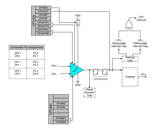
Figure 12.1. Comparator Functional Block Diagram
