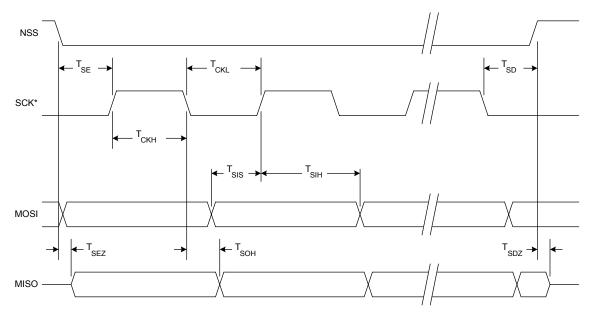
Figure 21.14. SPI Slave Timing (CKPHA = 0)
