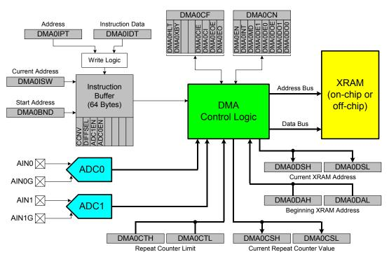
Figure 6.1. DMA0 Block Diagram
