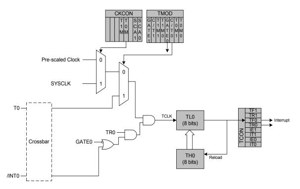
Figure 24.2. T0 Mode 2 Block Diagram
