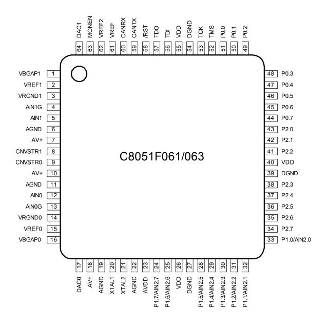
Figure 4.4. C8051F061 / C8051F063 Pinout Diagram (TQFP-64)
