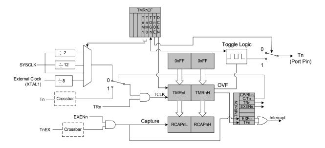
Figure 24.11. T2, 3, and 4 Capture Mode Block Diagram
