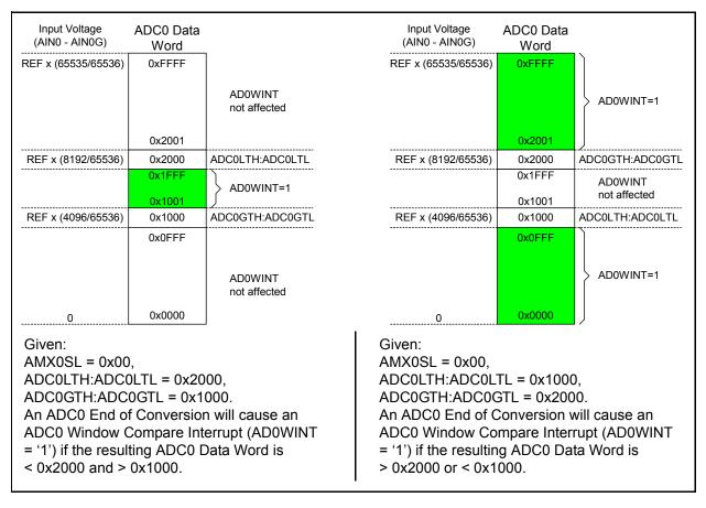
Figure 5.28. 16-Bit ADC0 Window Interrupt Example: Single-Ended Data
