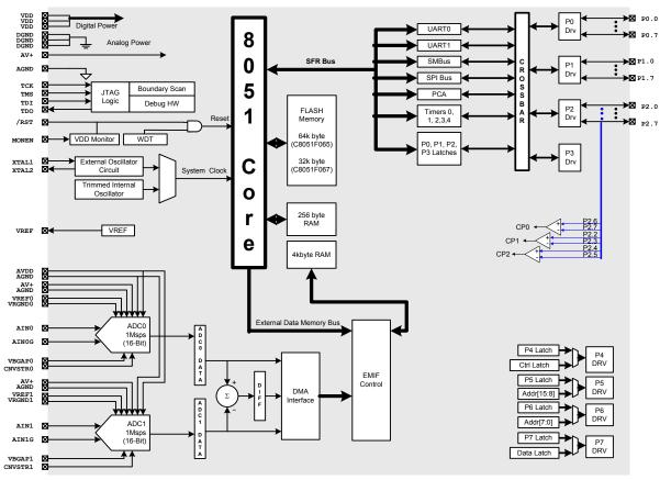
Figure 1.4. C8051F065 / C8051F067 Block Diagram
