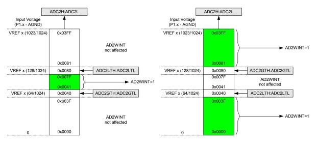
Figure 7.15. ADC Window Compare Example: Right-Justified Single-Ended Data
