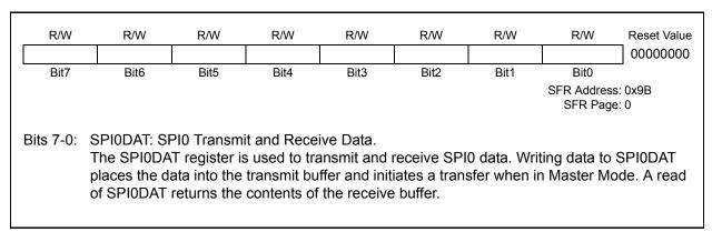
Figure 21.11. SPI0DAT: SPI0 Data Register
