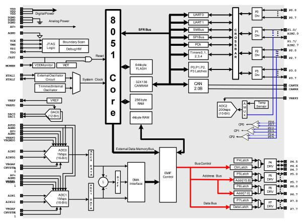
Figure 1.1. C8051F060 / C8051F062 Block Diagram
