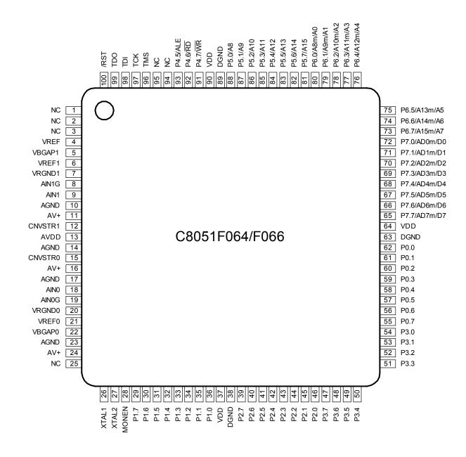
Figure 4.2. C8051F064 / C8051F066 Pinout Diagram (TQFP-100)
