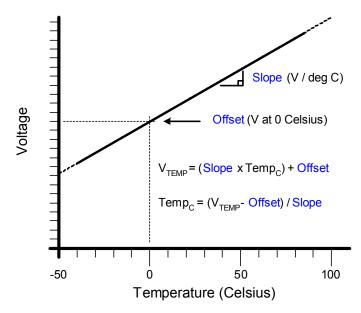
Figure 7.2. Temperature Sensor Transfer Function
