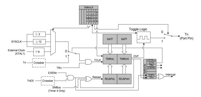
Figure 24.12. T2, 3, and 4 Auto-reload Mode Block Diagram
