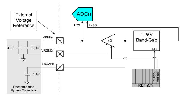
Figure 5.3. Voltage Reference Block Diagram
