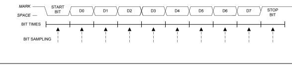
Figure 22.4. UART0 Mode 1 Timing Diagram
