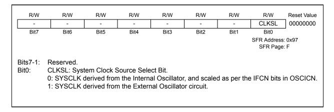
Figure 15.4. CLKSEL: Oscillator Clock Selection Register
