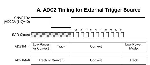
Figure 7.3. 10-Bit ADC Track and Conversion Example Timing
