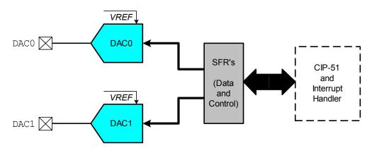
Figure 1.14. DAC System Block Diagram
