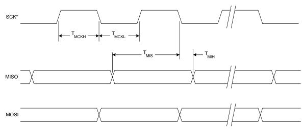
Figure 21.12. SPI Master Timing (CKPHA = 0)
