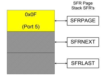
Figure 13.4. SFR Page Stack While Using SFR Page 0x0F To Access Port 5
