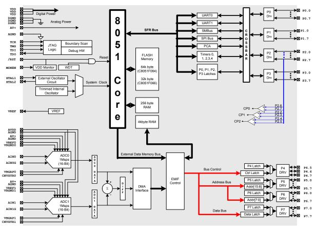
Figure 1.3. C8051F064 / C8051F066 Block Diagram
