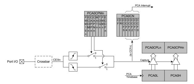
Note: The signal at CEXn must be high or low for at least 2 system clock cycles in order to be valid.
