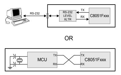
Figure 23.3. UART Interconnect Diagram
