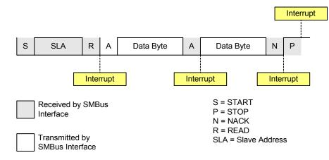
Figure 20.6. Typical Slave Transmitter Sequence
