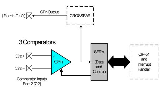
Figure 1.15. Comparator Block Diagram
