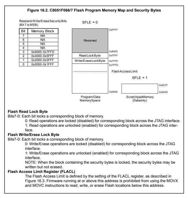
The Flash Access Limit security feature (see Figure 16.3) protects proprietary program code and data from being read by software running on the C8051F060/1/2/3/4/5/6/7. This feature provides support for OEMs that wish to program the MCU with proprietary value-added firmware before distribution. The value-added firmware can be protected while allowing additional code to be programmed in remaining program memory space later.
