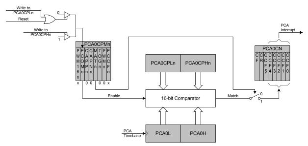
Figure 25.5. PCA Software Timer Mode Diagram
