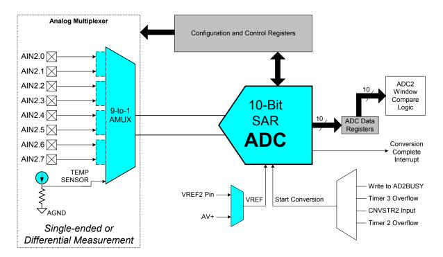
Figure 1.13. 10-Bit ADC Diagram
