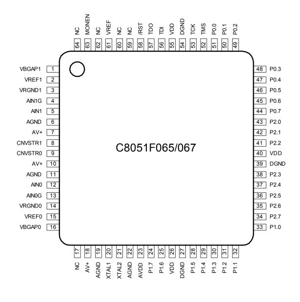
Figure 4.5. C8051F065 / C8051F067 Pinout Diagram (TQFP-64)
