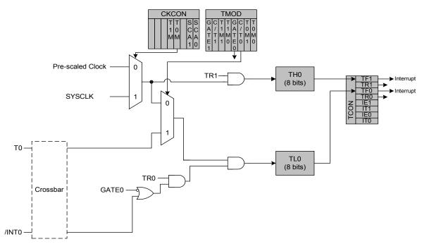
Figure 24.3. T0 Mode 3 Block Diagram
