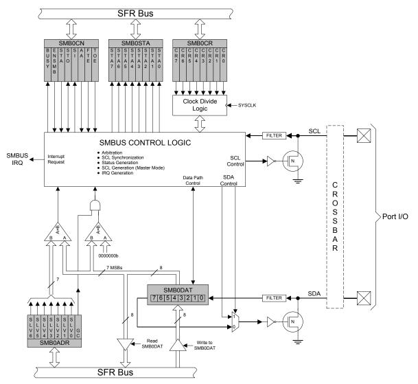
Figure 20.1. SMBus0 Block Diagram
