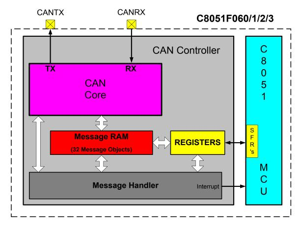
Figure 19.1. CAN Controller Diagram
