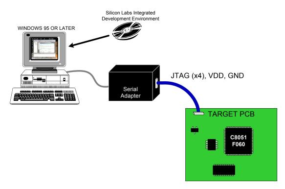
Figure 1.8. Development/In-System Debug Diagram
