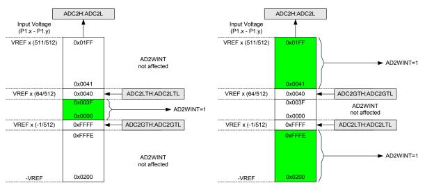
Figure 7.17. ADC Window Compare Example: Right-Justified Differential Data
