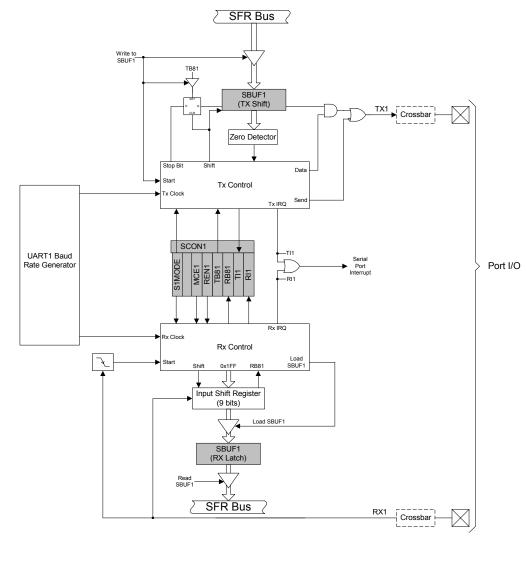
Figure 23.1. UART1 Block Diagram
