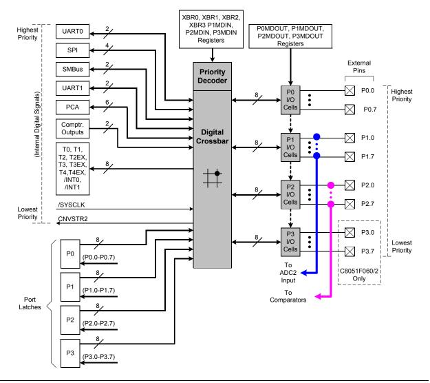
Figure 18.2. Port I/O Functional Block Diagram
