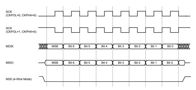
Figure 21.6. Slave Mode Data/Clock Timing (CKPHA = 0)
