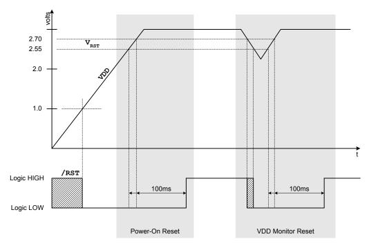
Figure 14.2. Reset Timing
