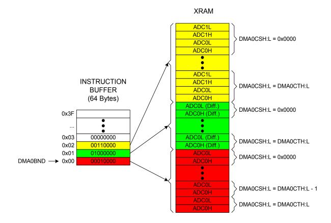
Figure 6.3. DMA Mode 1 Operation
