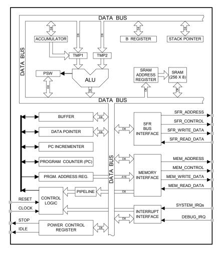
Figure 13.1. CIP-51 Block Diagram
