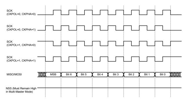
Figure 21.5. Master Mode Data/Clock Timing
