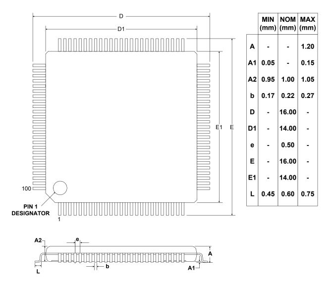
Figure 4.3. TQFP-100 Package Drawing
