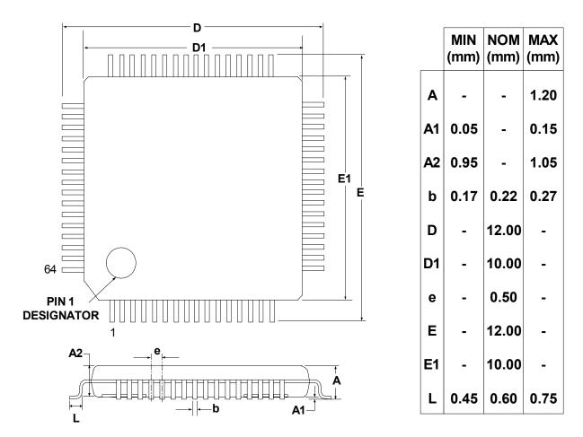
Figure 4.6. TQFP-64 Package Drawing
