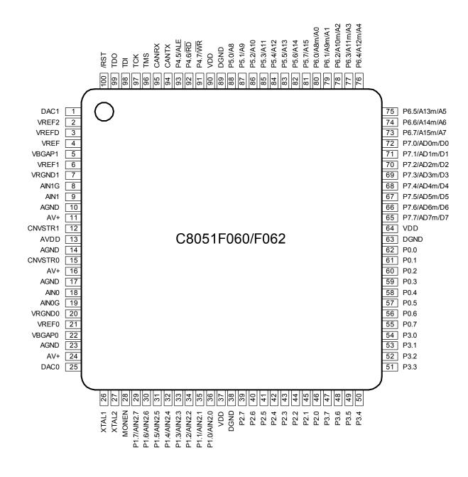
Figure 4.1. C8051F060 / C8051F062 Pinout Diagram (TQFP-100)
