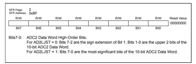
Figure 7.9. ADC2L: ADC2 Data Word LSB Register
