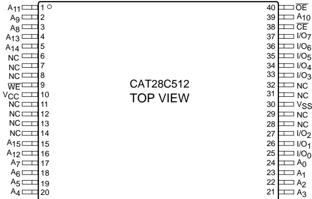
TSOP Package (10mm X 14mm) (T14)
