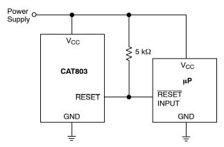
Figure 11. Typical CAT803 Open-Drain Circuit Configuration
