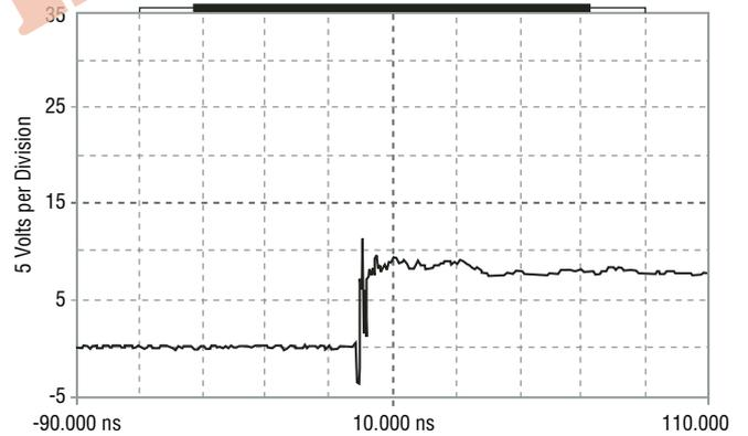
ESD Test Pulse - 25 kilovolt, 1/30 ns (waveshape)
