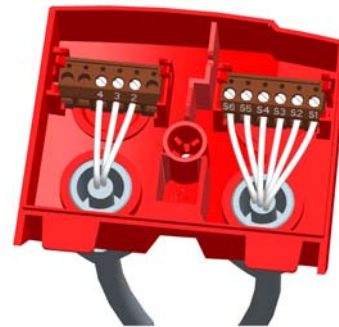
Fig. 8. Access cover (models with internal switches)
