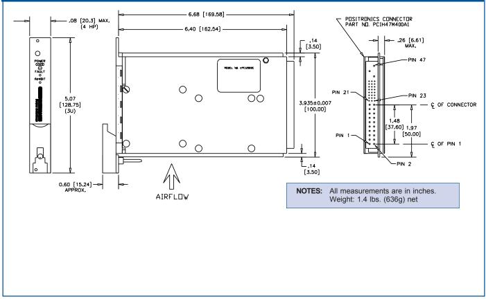
PIN ASSIGNMENT: Pin assignment consistent with PICMG™ 2.11R1.0 specification. The table below details the PICMG™ assignment.
