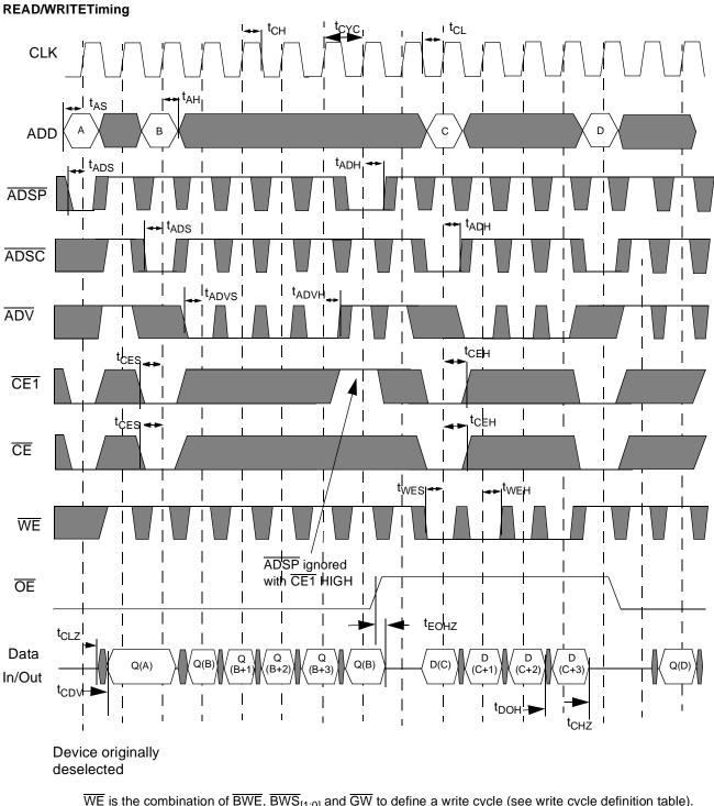
$\overline{\text{WE}}$  is the combination of  $\overline{\text{BWE}}$ ,  $\overline{\text{BWS}}_{[1:0]}$  and  $\overline{\text{GW}}$  to define a write cycle (see write cycle definition table).  $\overline{\text{CE}}$  is the combination of  $\text{CE}_2$  and  $\overline{\text{CE}}_3$ . All chip selects need to be active in order to select the device. RAx stands for Read Address X, WA stands for Write Address X, Dx stands for Data-in X, Qx stands for Data-out X
