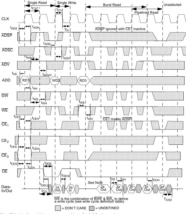
Note: Write data forwarded to outputs on read immediately following a write
