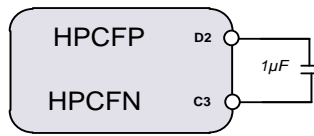
Figure 39: Charge pump flying capacitor
