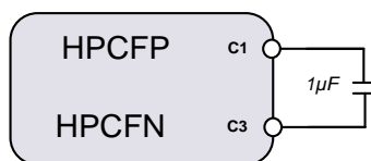
Figure 41: Charge Pump Flying Capacitor
