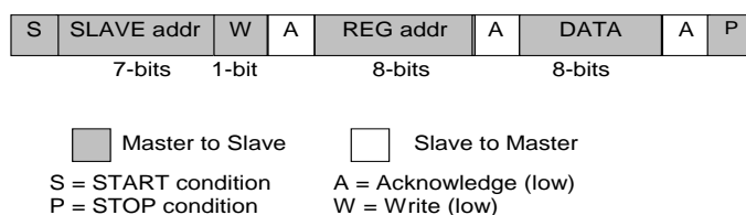
Figure 27: I 2 C Byte Write (SDA signal)
