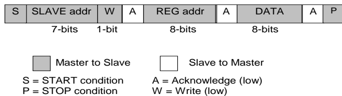
Figure 27: I 2 C Byte Write (SDA signal)
