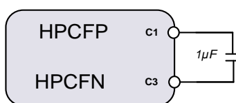
Figure 41: Charge Pump Flying Capacitor
