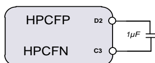
Figure 39: Charge pump flying capacitor
