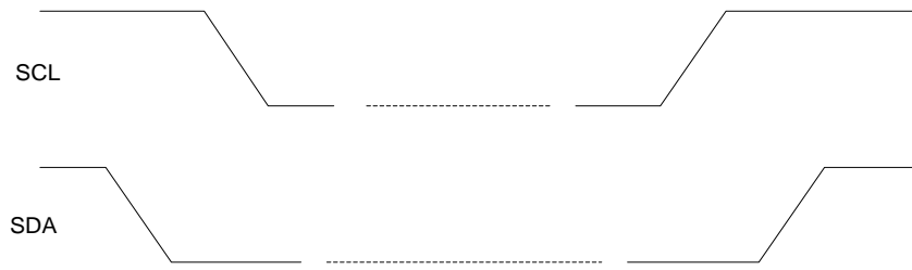
Figure 23: I2C START and STOP conditions
