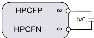
Figure 39: Charge Pump Flying Capacitor
