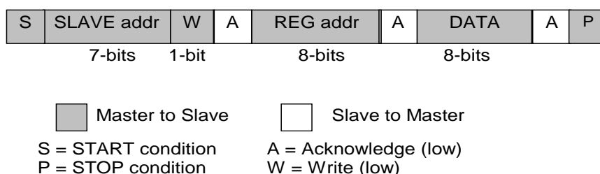
Figure 34: I 2 C Byte Write (SDA line)
