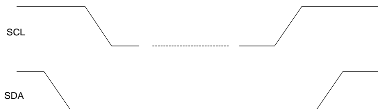
Figure 33: I 2 C START and STOP Conditions
