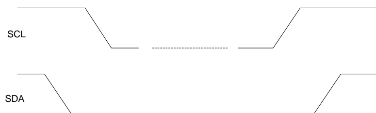
Figure 33: I 2 C START and STOP Conditions
