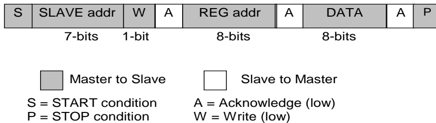
Figure 35: I 2 C Byte Write (SDA line)
