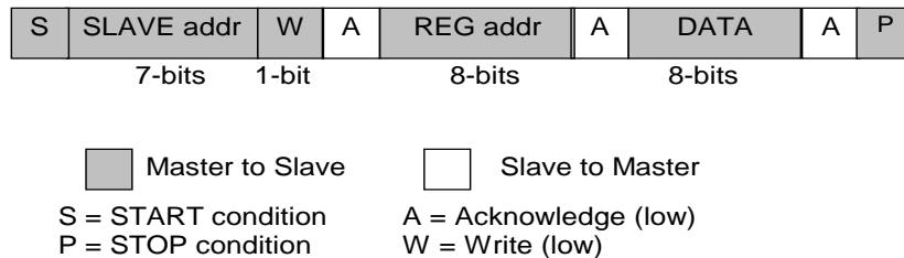
Figure 35: I 2 C Byte Write (SDA line)
