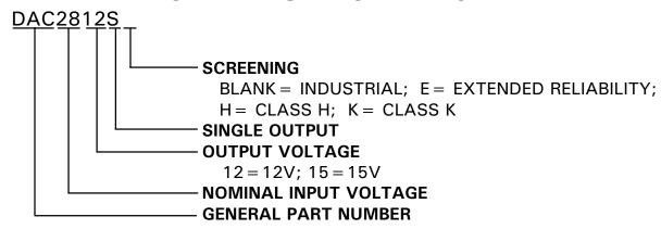
The above example is an industrial grade 12V single output converter
