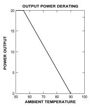
Typical Performance: (Tc=25°C, Vin=Nom VDC, Rated Load)
