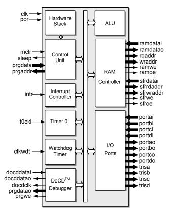
**Timer 0** – Main system's timer and prescaler. This timer operates in two modes: 8-bit timer or 8-bit counter. In the "timer mode", timer registers are incremented every 4 CLK periods. When the prescaler is assigned into the TIMER prescale ration can be divided by 2, 4 .. 256. In the "counter mode" the timer register is incremented every falling or rising edge of T0CKI pin, dependent on T0SE bit in OPTION register.
