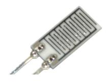
The EMD-4000 is a bulk resistance-type humidity sensor based on the impedance change of a thin-film polymer due to water vapor absorption. The polymer is deposited on Bismuth alloy terminals, which are set on a ceramic substrate. The sensor is excited by a low voltage alternating current and the impedance measured as a function of relative humidity.
